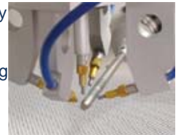
A microabrasive blasting system can be used to clean and prepare stent surfaces for electropolishing.
